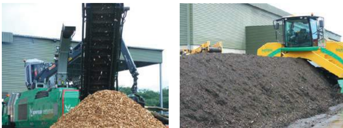
Figure 2.6 Mechanization has made large-scale composting possible: a drum chipper (left) and windrow turner (right).
