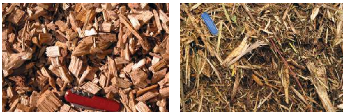
Figure 2.4 Wood chips (left) cannot be efficiently decomposed by compost microorganisms, whereas defibered wood (right) can. The use of defibered wood results in a better structure within the windrows and allows for a better aeration.
