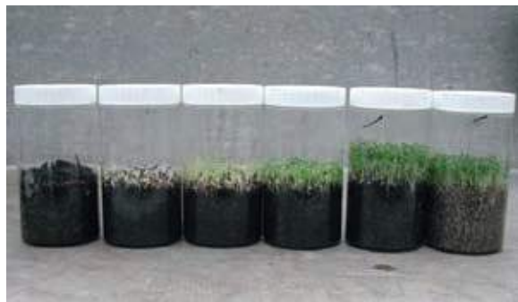
Figure 4.7 Phytotoxicity tests to assess the compatibility of composts with plants. Left: open cress test. Right: closed cress test.
